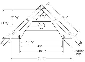
Figure 5 - Framing Clearances for Corner Installation
